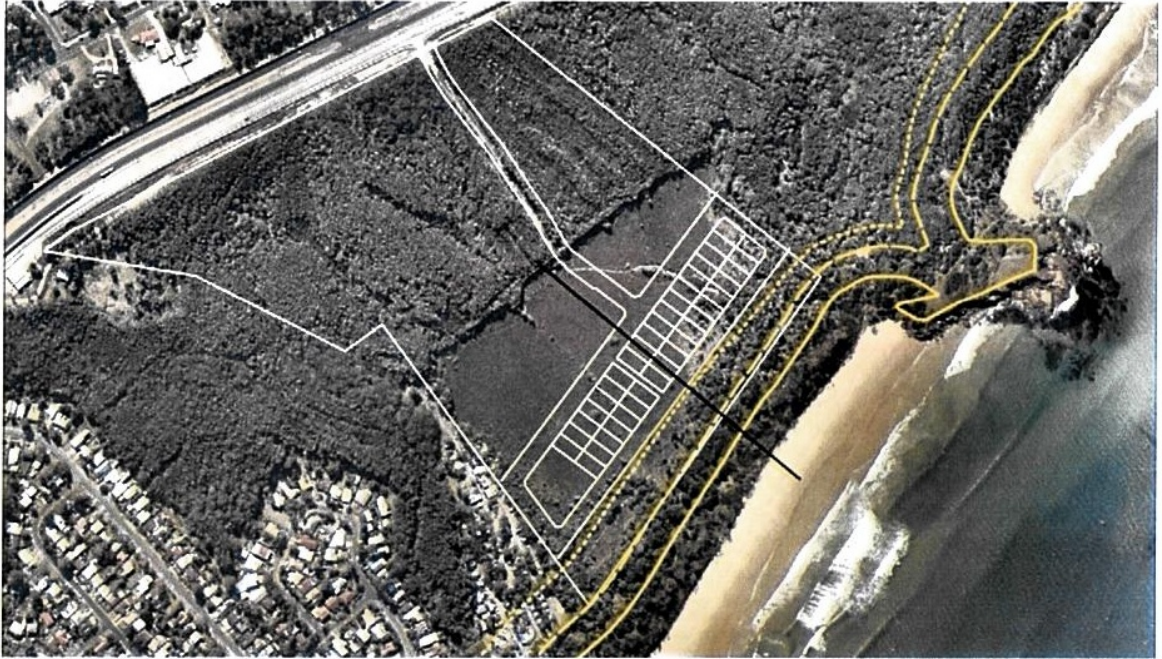
Figure 1: Cross section location for profile given in Figure 2, showing 'unlikely' 2010, 2050 and 2100 hazard lines (progressing landward) and the proposed development layout
