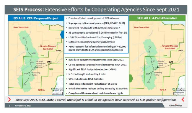
The light green polygons in the above image represent the maximum underground drilling reach from the small surface pads.
