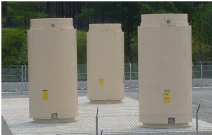
Transportable spent fuel storage casks sit on a storage pad. (Courtesy: Holtec International)
