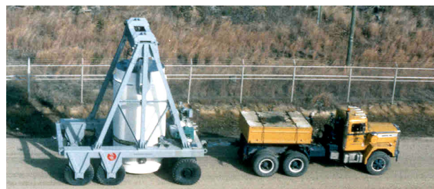
Cask transporter moves loaded spent fuel storage cask to storage pad.
